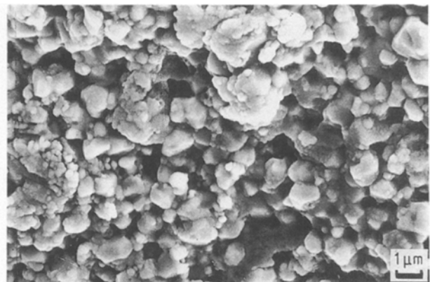
Figure 8 Fracture facies of a TiC 0.67 N 0.33 -21 vol % ZrO 2 composite sintered at 1550 °C.
